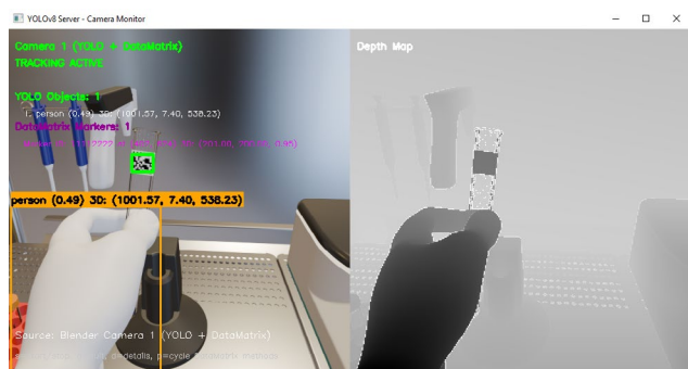
Figure 4 – Using a virtually generated camera feed in detection algorithms (object detection/tracking, 2D code reading)
